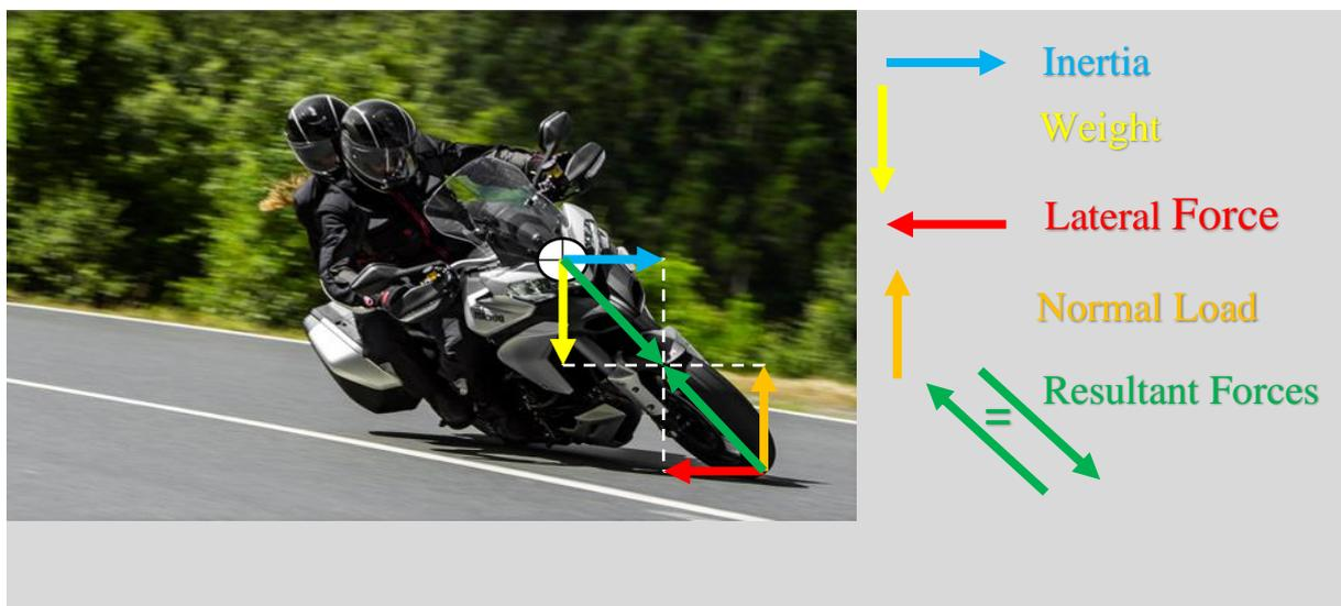
The Weight now exerts a Torque ( $T_1$ ) about the Contact Point. Torque is the ‘turning effect of a force’ and the size of the Torque is found by multiplying the Force by the offset distance from the point of application of the Force, to the point about which it tries to rotate the bike. The size of  $T_1$  is therefore the product of the Weight of the bike and rider and the offset distance to the Roll Axis:
