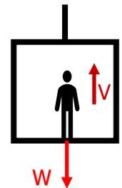
1. When the lift begins to move from the ground floor, it accelerates upwards, as shown by the blue arrow. The Inertia Generated Force (green arrow) opposes the acceleration and acts in the same direction as the man's weight (red arrow), which makes him feel heavier, with an apparent weight of  $(W+I)$  during the acceleration phase.
