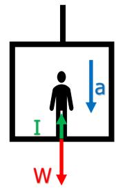
2. Between floors there is no acceleration and the lift travels upwards at constant velocity, as shown by the brown arrow. If there is no acceleration, there is no Inertia Generated Force and the man feels his correct weight (W).
