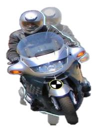
Pushing away gently on the **Right** handlebar end, makes the bike go to the Right.
