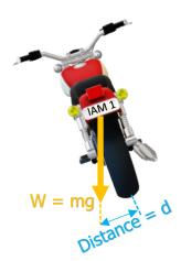
To find the 'direction' of the Camber Torque, we need to apply the Right-hand Rule I.E. curl the fingers of the right hand and point them in the direction of the roll; the right thumb then points in the direction of the Torque, in this case Camber Torque (T<sub>c</sub>)
