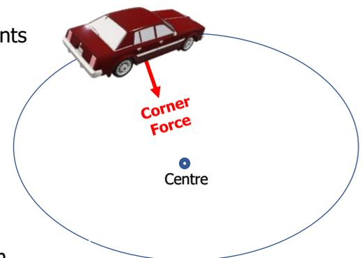
**Corner Force** is a demand that must be met and the force that primarily meets this demand is the **Friction Force** (I.E. also referred to as 'Grip') between the tyres and the road surface. If there is enough **Friction** to meet the **Corner Force** demand, the car remains stable in the bend; but if the **Corner Force** demand exceeds the maximum amount of Friction available, the car will Understeer in the bend and run wide: which has serious safety implications!
