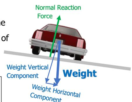
**In the case of a racing car** on a banked circuit, the additional **Horizontal Weight Component** acting down the slope effectively **increases** the amount of **Corner Force** demand the car can cope with, before Understeer starts: which means that the racing car can go through the bend faster, than it would be able to on a flat track with the same bend radius. I.E. greater speed results in greater Corner Force.
