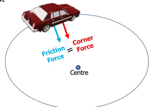
Banking a bend in the way described above, results in some of the car's Weight acting down the slope, in the direction of the centre of the bend. Consequently, this component of the car's weight adds to the Friction Force and helps it to meet the Corner Force demand.
