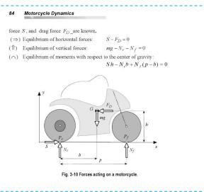
By lowering your torso on to the tank, the height of the combined bike / rider Centre of Gravity is reduced (I.E. h gets smaller).
