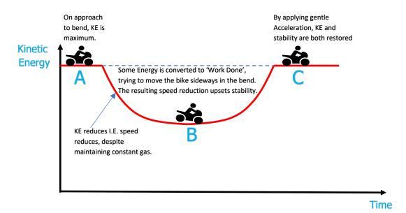
At Point A in the diagram above, the rider approaches the bend at a fixed and appropriate Velocity. Kinetic Energy is proportional to the square of the 'Speed' element of the bike's Velocity. For this manoeuvre, we can take this initial Kinetic Energy to be the maximum Kinetic Energy; although the term is purely relative and does not imply an *absolute* maximum value of Kinetic Energy.
