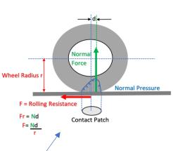
multiplied by the Radius of the wheel: as shown in the diagram above.
