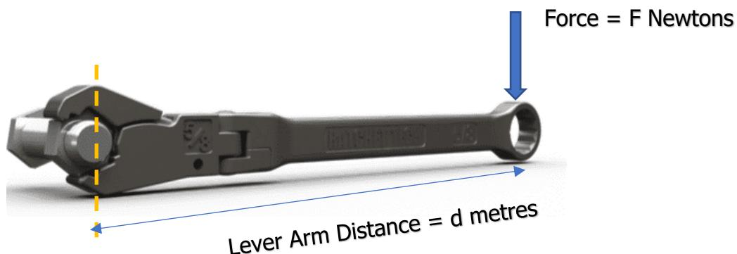
$$\text{Torque} = F \times d \text{ Newton metres}$$
