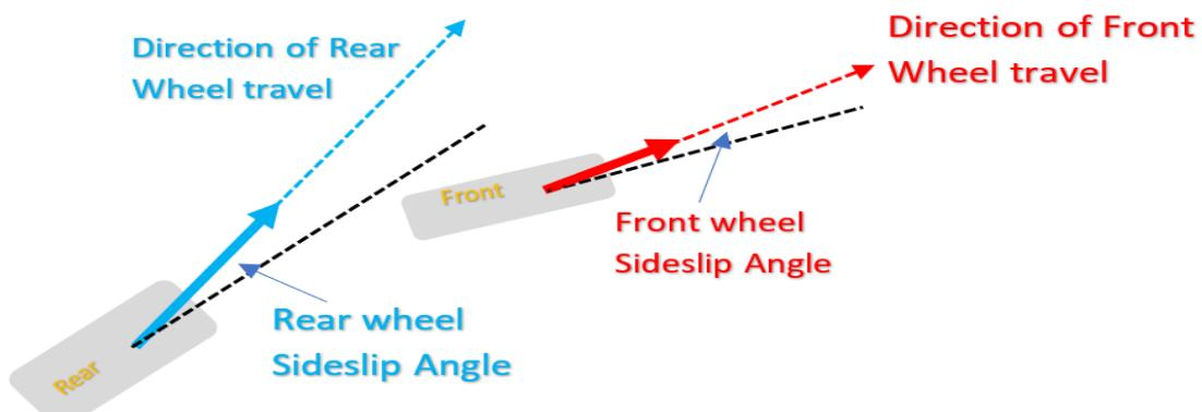
The Driving Force, also known as the Traction Force, and the Rear Wheel Braking Force are both applied at the rear wheel Contact Patch: there is no Traction Force applied to the Front Wheel Contact Patch, although the Front Wheel Braking Force is applied there.
