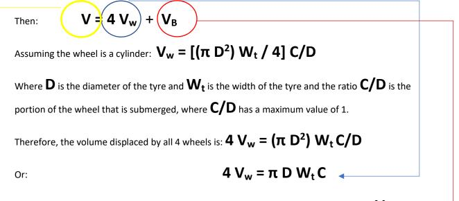
Now for the volume of the submerged part of the vehicle at the point at which it floats  $old V_B$
