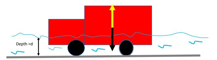
The vehicle will float when the **Upthrus**t (shown by the yellow arrow) is equal to the **Weight** of the car (shown by the black arrow)
