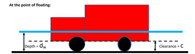
Volume of displaced water (V) = Volume displaced by the wheels + Volume displaced by the body.
