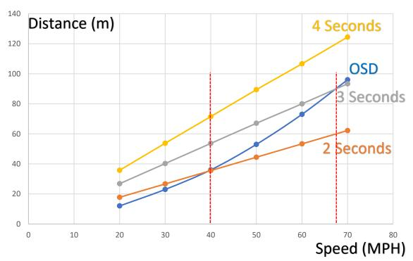
**For speeds below 40mph**, a 2 second gap gives a following distance which is more than the Overall Stopping Distance from the vehicle ahead, in compliance with HC Rule 126.
