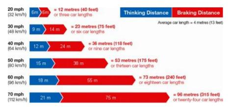
**Thinking Distance** is the distance travelled by the driver during the time it takes to react and before applying the brakes. It increases linearly with speed and assumes that **Reaction Time** will be the same irrespective of the speed at which you are travelling. Everyone is different and our Reaction Times can vary from day to day, but the Table assumes an average Reaction Time of 0.675 seconds, which is reasonable for the population of drivers in general.
